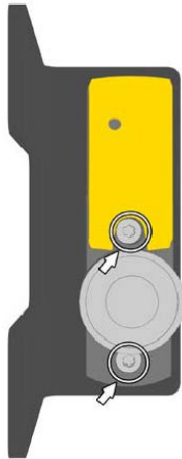
Fig.7: Attach the process guard locking to the mounting plate and tighten the Torx screws M6 x 25 mm.
