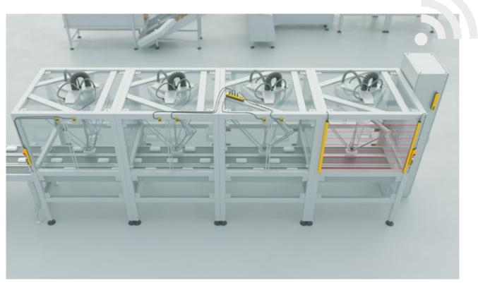
Implementation of safety technology with wireless safety on an assembly plant.
