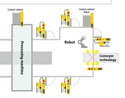
Automated processing machines often have a complex safety system, the emergency stop buttons switch off the entire plant. Material loading and unloading is provided with safety light grids, with or without muting. Safety switches with guard locking secure the service doors of the plant. Areas that can be stepped behind are unlocked with a pre-reset button. Thanks to the Safety Simplifier, the planning, extension and commissioning of safety technology can be significantly reduced.
