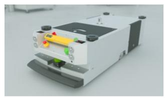
With the Safety Simplifier, automated guided vehicles can be switched off safely and wirelessly. Safe networking to production plants is possible at any time.
