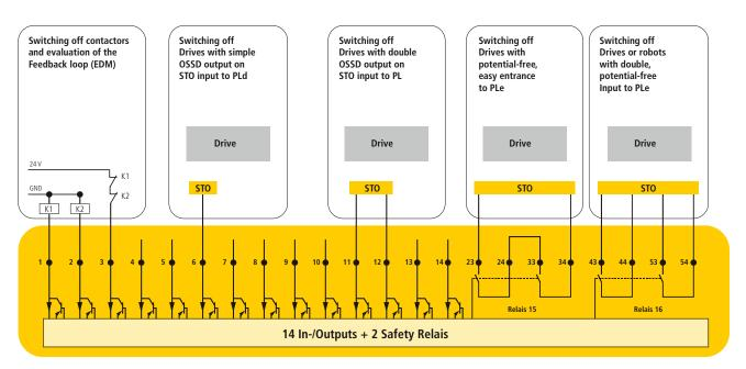
Connection example, safe outputs to Safety Simplifier S16
