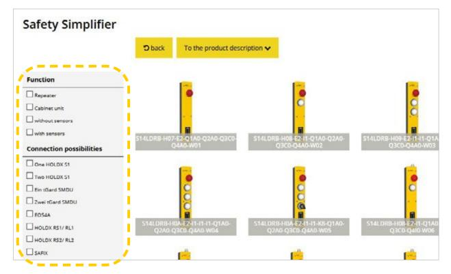
Plug & Play: The pre-wired Safety Simplifier standard variants can be directly connected and used. With the help of pre-configured connection options for safety solutions, such as safety switches or curtains, a plant can be put into operation in the shortest possible time without any wiring effort.
