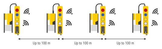
With the Safety Simplifier, very large ranges can be realized. The range between two participants is up to 100 meters. The integrated repeater function effectively extends the range. Safety Simplifier repeater modules can also be integrated to increase the range or to optimize the mesh network.
