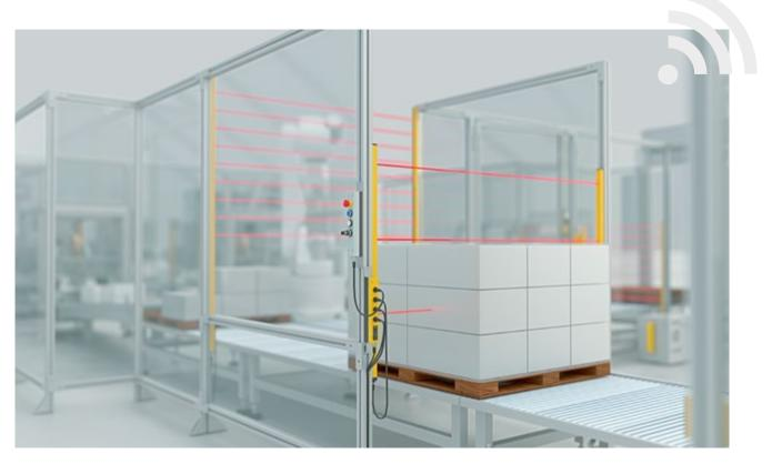
Safety Simplifier interlocking function with EOS4 light grids for unloading of pallets
