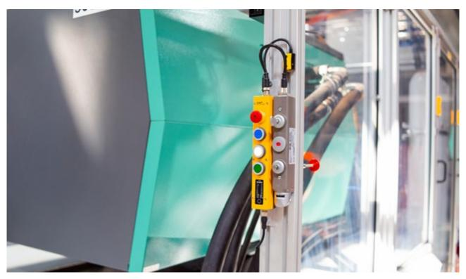
Safety Simplifier with Euromap interface on an injection molding machine.
