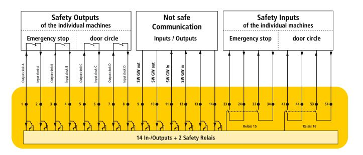
The Safety Simplifier on a single machine, mounted on the control cabinet, handles safe but also non-safe communication for the linking of the plant.
