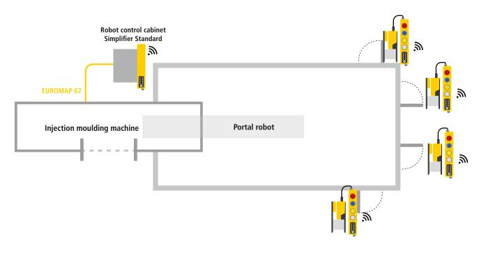
Example of an injection molding plant with Safety Simplifier
