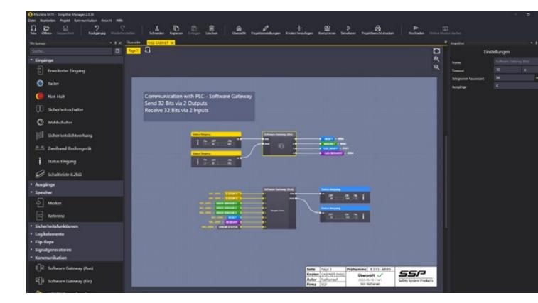
Communication with the Siemens PLC from the Simplifier Manager
