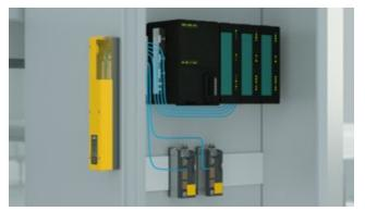
External mounting on the control cabinet saves space. Thanks to the LED display, diagnosis can be done without opening the control cabinet.
