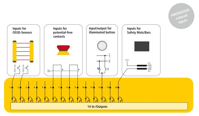
Connection example, safe inputs to the Safety Simplifier S14
