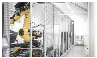
Stable spot welding grid with reinforcing fixation technology and robust aluminum profiles. SSP safety fences are regularly tested using pendulum and ballistic tests.
