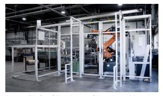
The route of the fence follows the route of the machine and the application. Angles, slopes, fillings and much more can be customized with the Flex-Line model.
