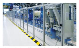
Thanks to polycarbonate fillings, the machines stay perfectly visible and provide not only grip guard and protection, but also good-looking machine safety.
