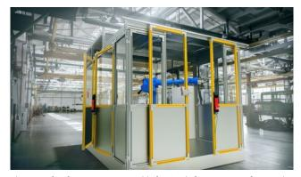
The SSP safety fence system is suitable for simple fence sections, for complex machine enclosures and for the enclosures of robotic installations, machines and manual workstations.
