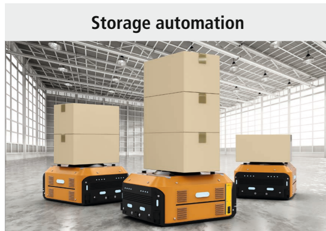
Thanks to the wireless interface, the vehicles can be switched off safely with an external emergency stop button.
